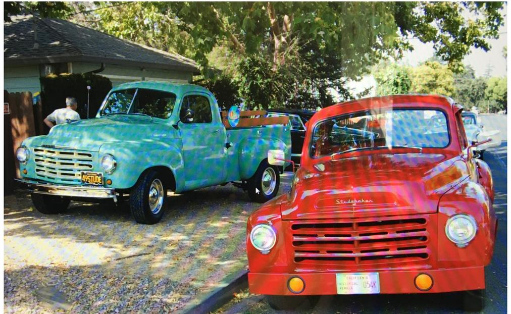
the center one. You can also clearly see that there are no slots punched through under the lower grill openings. They are impressed into the metal but are not cut through. I used to think Studebaker used the old 2R grills but no. I'm sure they saved a little bit of money on the newer version.
