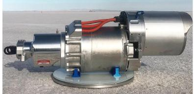
fornia, has unveiled their own Tesla crate motor for muscle EV conversions: As you can see, it's an entire Tesla drive unit with power inverter and the brackets to be mounted like a block motor.
