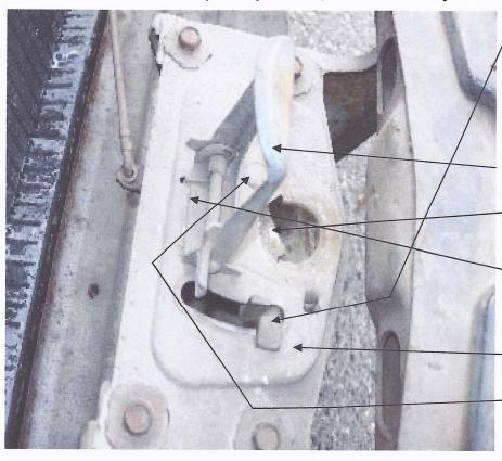
A - Lever and linkage to release primary and secondary hood latches.
